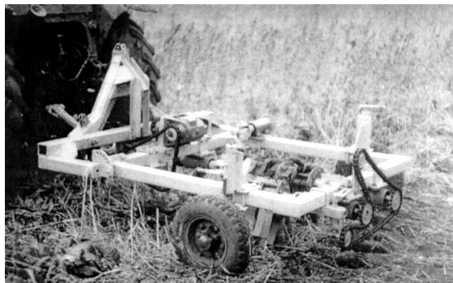
Fig. 2. General view of the experimental setup with a two-shaft cleaner of root crops heads from remains of tops
